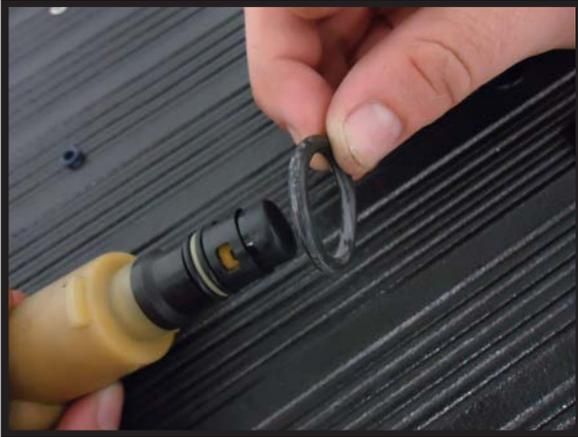
6. Apply a thin layer of o-ring lubricant and install the solenoid into the air spring in the reverse order of removal.
