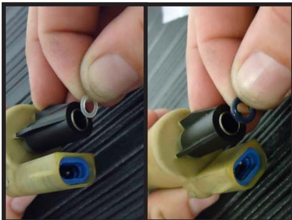
4. Stretch the o-rings out of the o-ring groove and off of the solenoid. **Be very careful not to damage sealing surfaces.**
