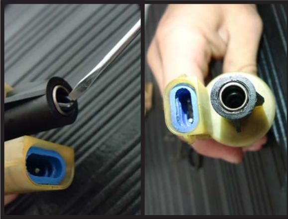
2. Insert the brass collet back into the solenoid. You will need to compress the bottom of the collet while you press it back into the opening. **Be very careful not to bend or distort the collet.**
