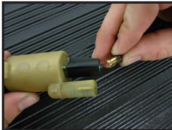
3. Remove the nylon washer and small o-ring.
