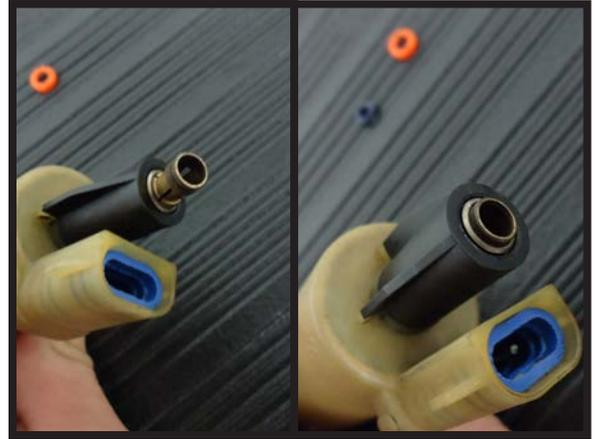
3. Once the collet is reinserted, press the orange collar top back over top of the collet making sure it snaps back into place.
