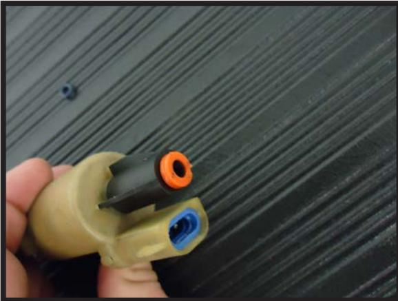
4. Roll the first o-ring over the tip of the solenoid and into the first o-ring groove. Do the same for the second o-ring stretching over the first o-ring already seated, and placing it into the second o-ring groove.
